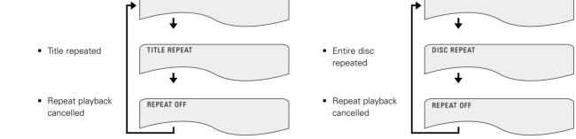
\* To return to normal playback: Return to normal playback by pressing the REPEAT button until "REPEAT OFF" appears on the TV screen.
